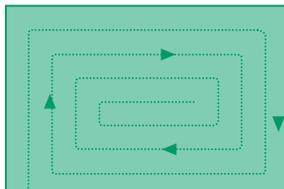
**Drop Spreader:** First make two passes along the top of the area you'll be covering. Then make two passes along the bottom area. Then move back and forth along the long part of the lawn. On each pass, as you reach the strips at the top and bottom of the area to be covered, shut off the spreader. It's also important to shut off the spreader when you are stopped.
